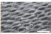
Scanning electron micrograph of the textured surface of the depressed areas on Stenocara surface.
